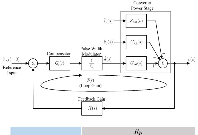
$H(s) - \text{feedback gain} \qquad \qquad \overline{R_a + R_b}$
