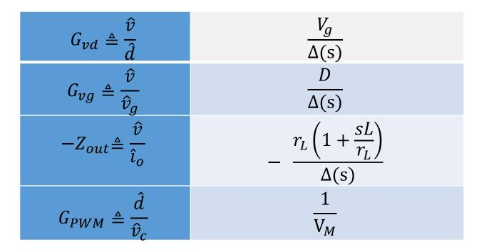
$$\Delta(s) = 1 + \frac{s}{\omega_0 Q} + \left(\frac{s}{\omega_0}\right)^2, \quad Q = \frac{\sqrt{LC}}{r_L C + \frac{L}{R}}, \quad \omega_0 = \frac{1}{\sqrt{LC}}$$
