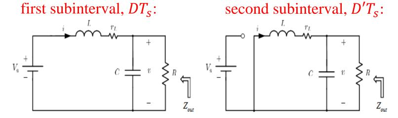
$$Z_{out} = (sL + r_L) \parallel \frac{1}{sC} \parallel R$$
